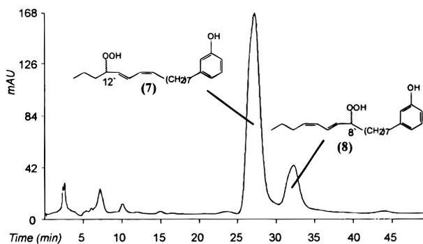
**Figure 4.** Normal phase HPLC separation of hydroperoxides formed by LOX-1-catalyzed dioxygenation of 3-[(*Z,Z*)-8',11'-pentadecadienyl]phenol (**1**). Product separation was performed on an Eurospher Si 100 column (250 × 4 mm, 5 μm); flow, 1 mL/min; eluent, pentane + ethanol = 100 + 1, monitored by UV detection at 234 nm.
