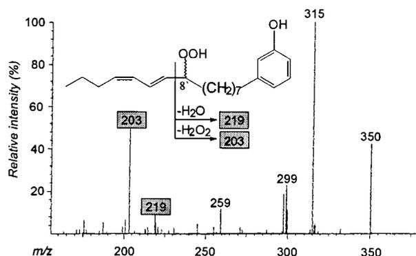
**Figure 6.** Product ion spectrum of 3-[8'-hydroperoxy-(*Z,E*)-9',11'-pentadecadienyl]phenol (**8**), precursor ion  $m/z$  350  $[M + \text{NH}_4]^+$  (ESI positive mode,  $-7$  eV, 0.24 Pa of argon as collision gas). Inset: fragmentation pattern explaining the characteristic ions observed.
